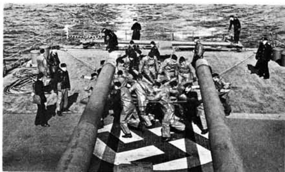
Steering the ship by operating the jury rudders by capstan power. The wires leading through leading-blocks to the rudder yokes can be clearly seen
