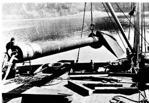
Huacarán. Two emergency rudders are constructed, fitted and operated through the stern capstan
