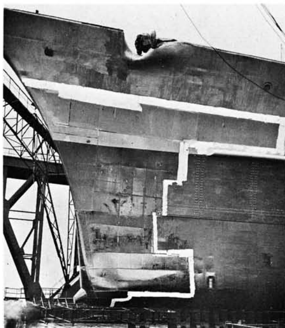
The new bow section is outlined in white. Note mines spar protuberance
